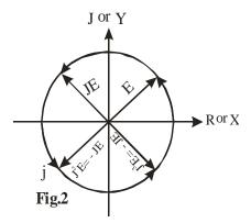
For vectors which rotates about some fixed point in a plane (called phasors), this concept of 'j' leads to a neat and simple algebraic way of performing vector operations.
